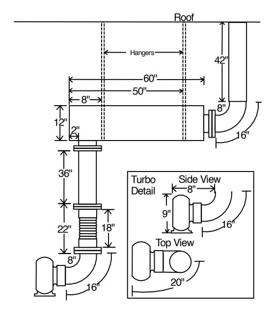
On elbows inside radius and outside radius measurements are best measured from welded seams or flanges.
